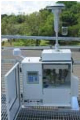
The Partisol aerosol sampler for measuring particulate air pollution on the roof of building 18 at CDU
